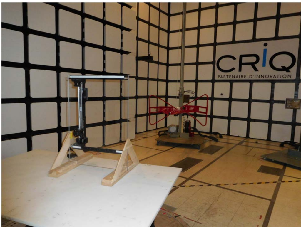
Measurement of radiated emissions: Test setup
